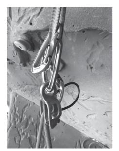
Step 2: Place a biner (does not have to be locking) on the focal point next to your belay device, on the side where the live rope (the rope going to the climber) and dead rope come out of the belay device.
